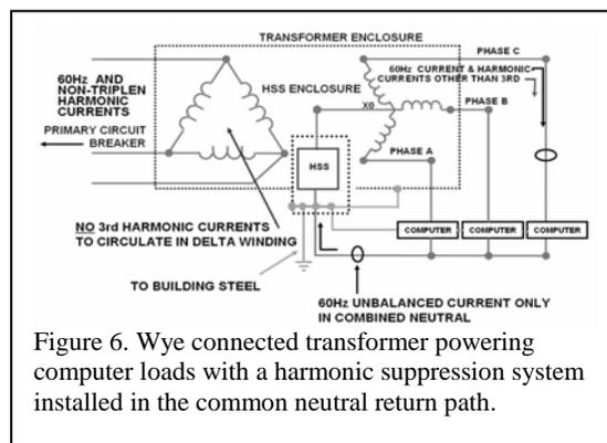
Figure 6. Wye connected transformer powering computer loads with a harmonic suppression system installed in the common neutral return path.
