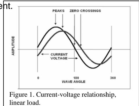
Figure 1. Current-voltage relationship, linear load.
