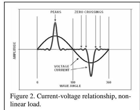
Figure 2. Current-voltage relationship, non-linear load.
