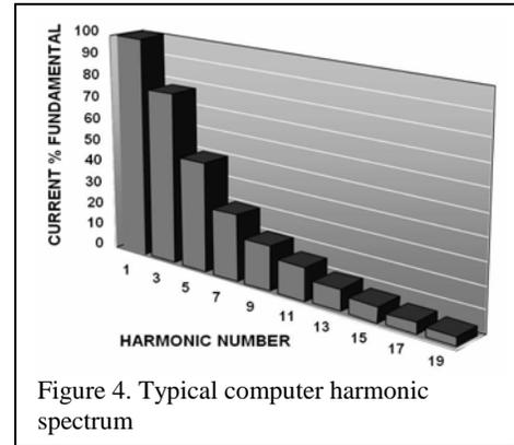
Figure 4. Typical computer harmonic spectrum
