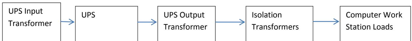
Removing the triplen 3<sup>rd</sup> harmonic component means less heat wasted in kWh in the transformer and the power distribution system as well as in the UPS filters, inverter and rectifier.
