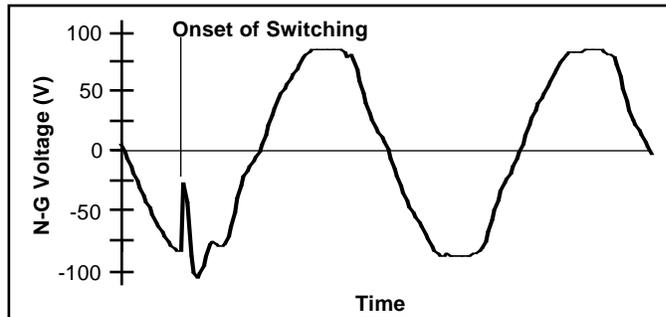
Figure 4. Neutral-to-Ground PC Voltage During Capacitor Switching
