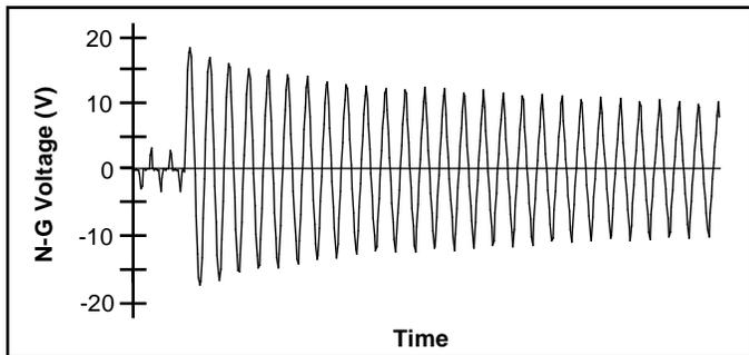
Figure 2. Neutral-to-Ground PC Voltage During Switching of Photocopier Heating Element (Long Branch Circuit)
