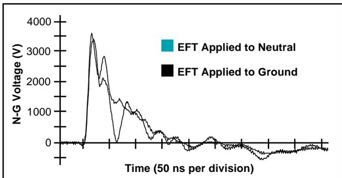
Figure 3. Neutral-to-Ground PC Voltage During Application of 4-kV Electrical Fast Transient
