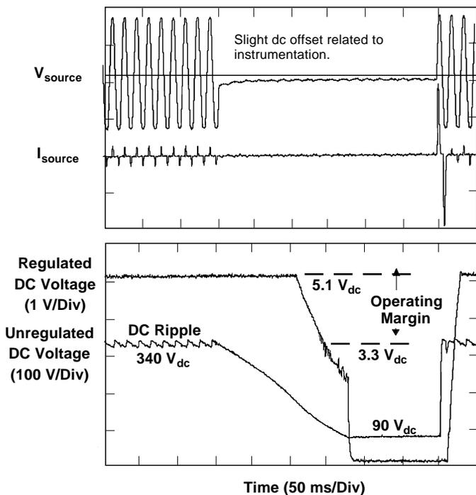
Figure 2. Unsuccessful Ride-Through During Momentary Interruption of Supply Voltage
