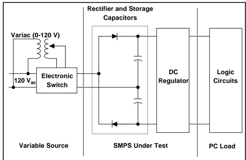
Figure 1. Diagram of Test Setup
