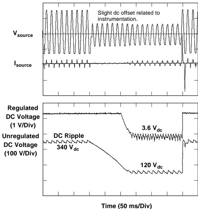
Figure 3. Successful Ride-Through During Voltage Sag to 50% of Supply Voltage
